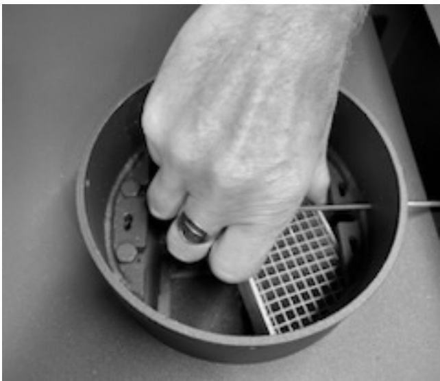
Figure 4: Rotate combustor under thermocouple.
