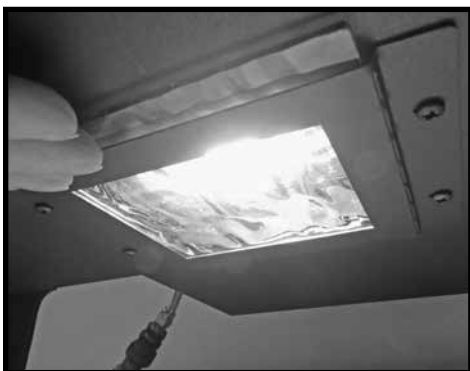
Figure 64: Glass plate holder access.
