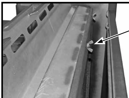
Figure 40: Door wing bolts.
