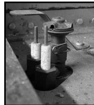
Figure 74: TN24 Pilot assembly.
