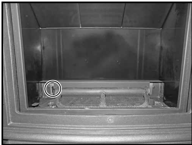
Figure 45: Burner with basket for embers. Tab located on left side of burner for #3 log placement.
