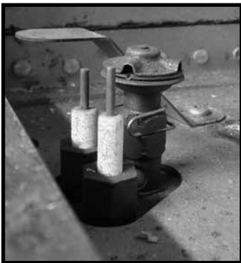
Figure 71: TN24 Pilot assembly.
